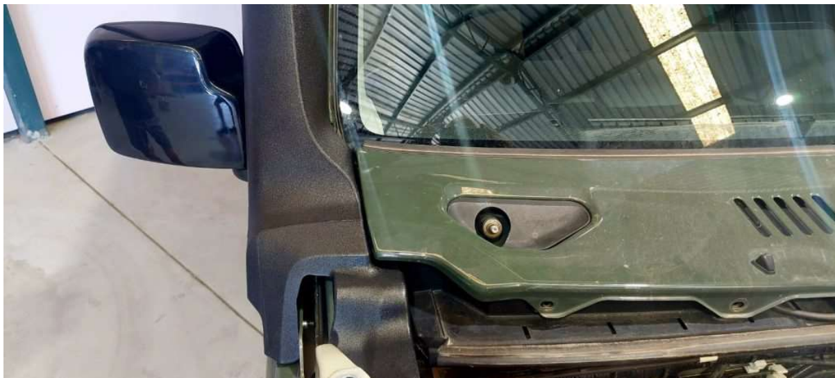
Suzuki Jimny Bravo Snorkel Installation Guide- Refit plenum panel
