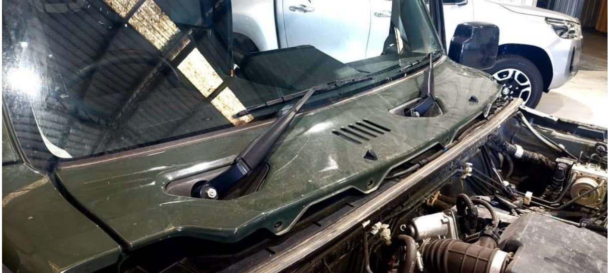
Suzuki Jimny Bravo Snorkel Installation Guide - remove the Plenum Panel 1
