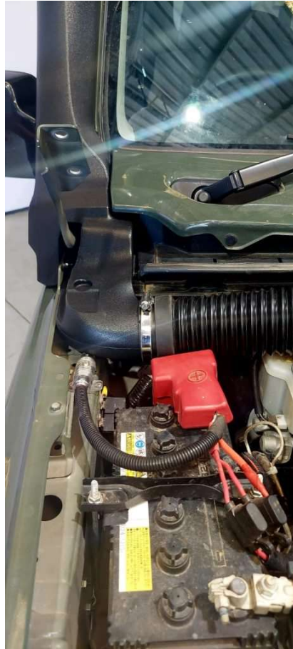
Suzuki Jimny Bravo Snorkel Installation Guide- Install airpipe 1
