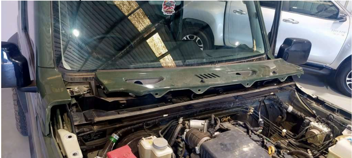
Suzuki Jimny Bravo Snorkel Installation Guide - remove the Plenum Panel 2
