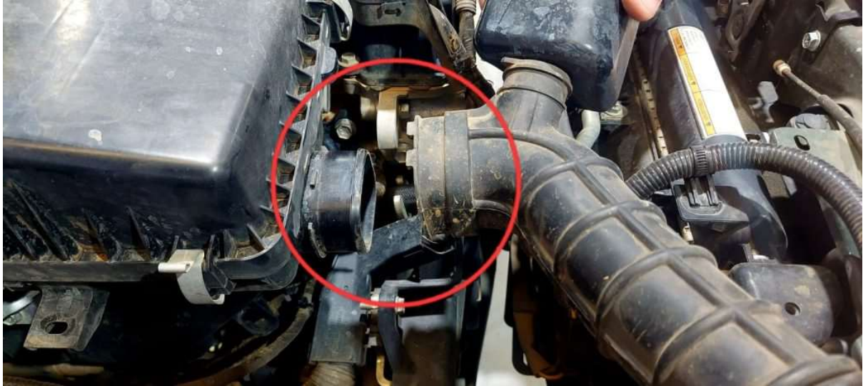
Suzuki Jimny Bravo Snorkel Installation Guide - Remove existing air intake pipe
