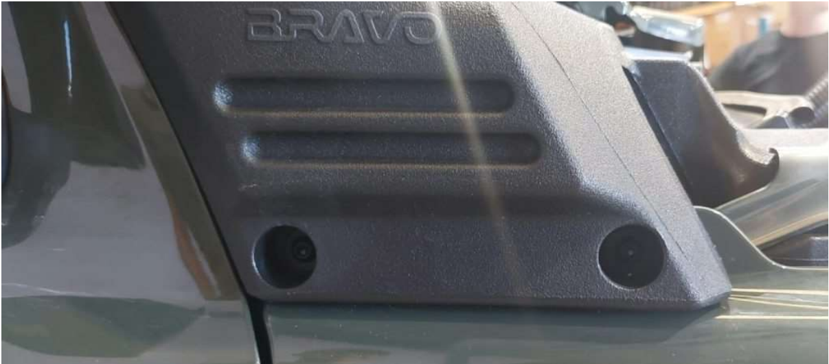
Suzuki Jimny Bravo Snorkel Installation Guide - Drill Hole in fender 1
